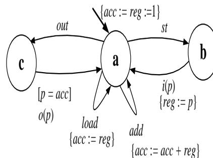
Fig. 2. ELTS model of the calculator
